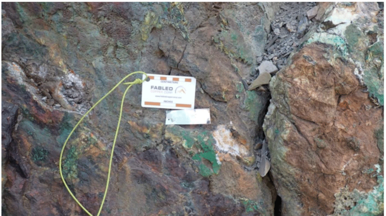
Chip Sample # D – 723424, elevation 1,457 m, 1.56% Copper over 0.50 meters
