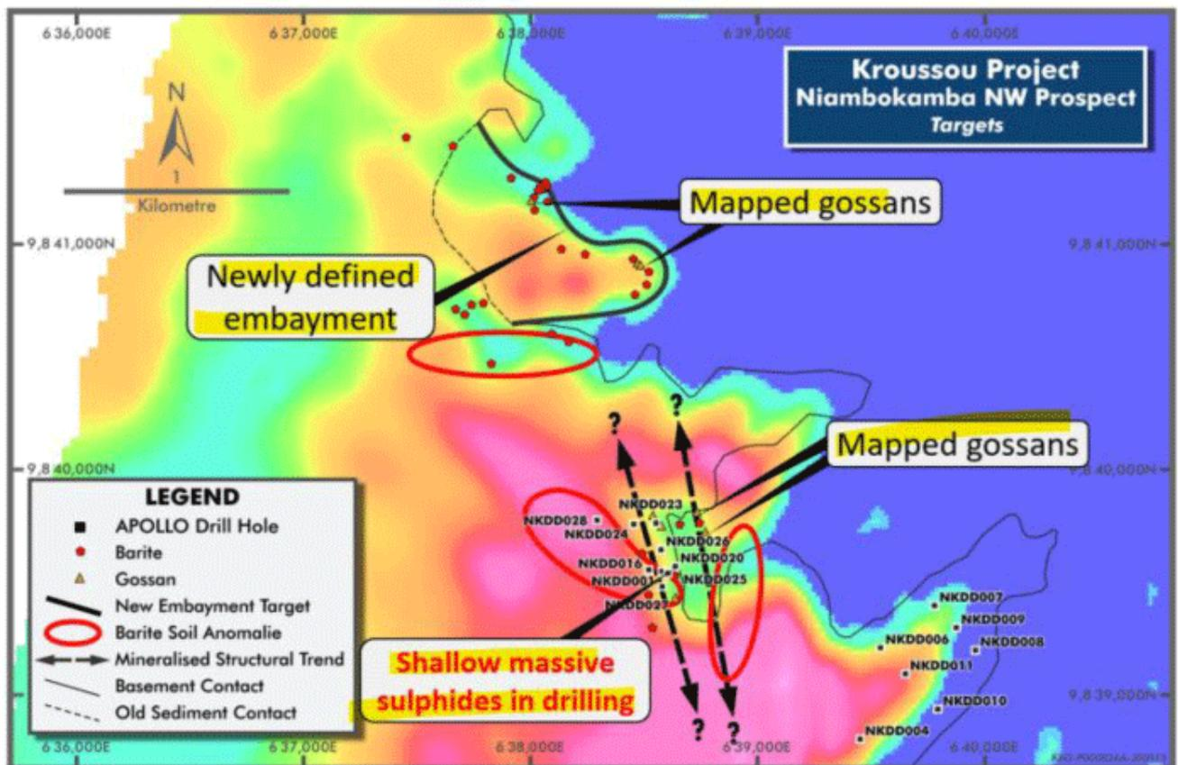
Figure 2: Newly identified embayment target and mapped gossans near TP13 NW (airborne EM data early time underlay).
