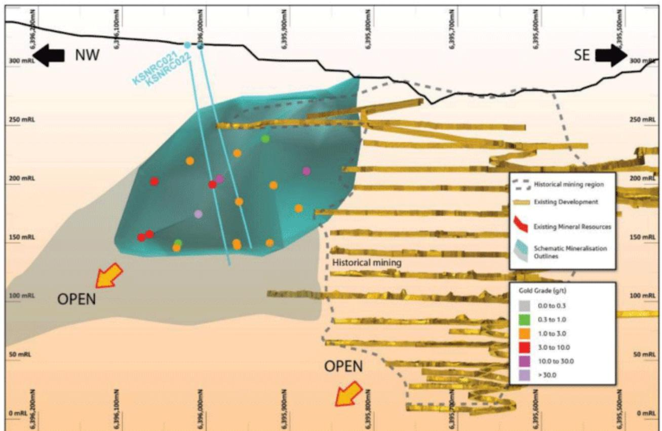
Figure 1: Long section view of Eastern Ore Zone (EOZ) showing extension potential.
